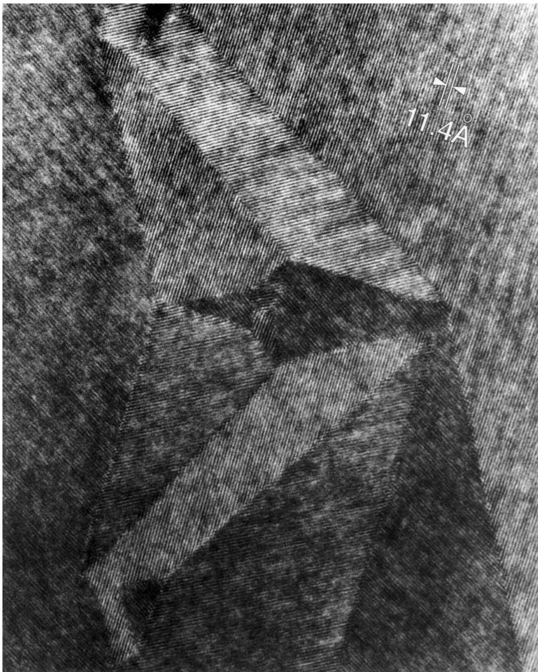
FIG. 13. Domain configuration exhibiting a fan pattern and a star pattern, imaged by the LPSS fringes.
